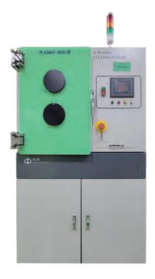
The Plasmax 800 series represents a batch-type plasma cleaning machine specifically designed for ion bombardment applications, aimed at enhancing the surface hydrophilicity prior to wire-bonding or molding processes to improve the process performance.
